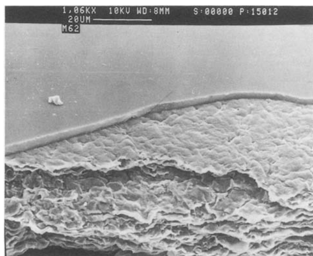
Photomicrograph 1. SEM image of a Na-montmorillonite/18C6 film coated by a PB layer of 5 \mu\text{m} thickness
